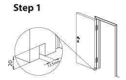
Machine a slot in the bottom of the door measuring 12.5mm wide x 20mm deep.
