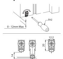
Adjust to suit under door gap using a Phillips screwdriver (PH2)
